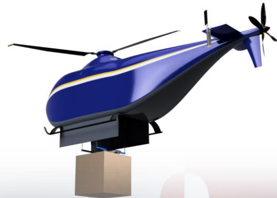
(6) Package is hoisted down
