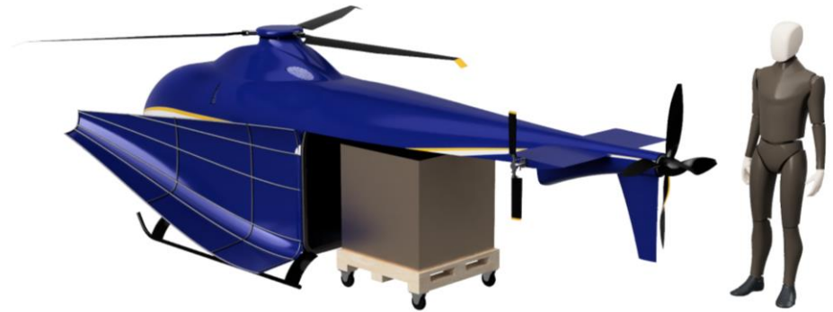
(2) Package is loaded using the variable height cart
