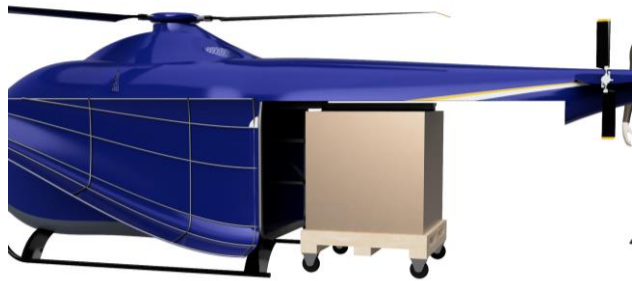
(3) Package is engaged in the low-friction rail and pushed inside by the operator
